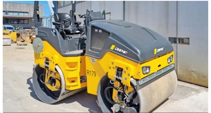
LE BOMAG BW 138 AD-5, 4'400 KG, EST UN ROULEAU TANDEM LÉGER PARFAIT POUR LE COMPACTAGE DES SOLS ET LES POSES D'ASPHALTE.
