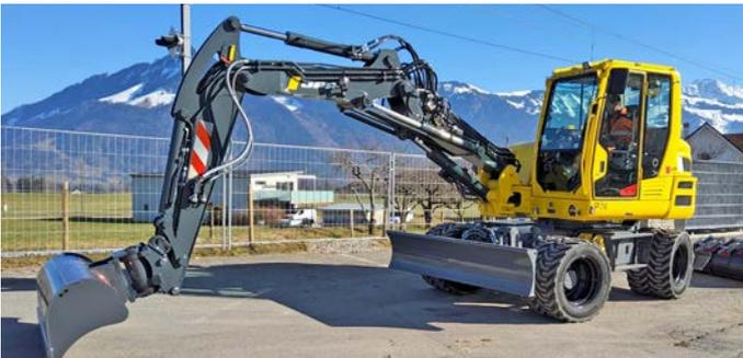
DEUX EXCAVATRICES SUR PNEUS TAKEUCHI TB395W 4WS RENFORCENT LA FLOTTE JPF, EN VERSION QUATRE ROUES DIRECTRICES ET PATTES.
