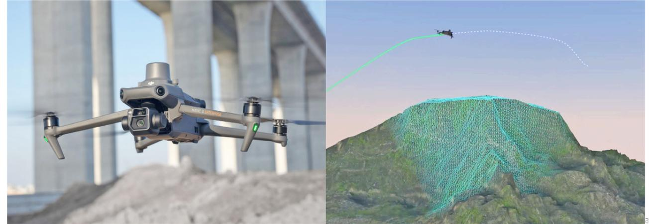
LE BUREAU DES GÉOMÈTRES COMPTE UN NOUVEAU DRONE DJI MAVIC 3 ENTERPRISE. IL PORTE LA PRÉCISION DES RELEVÉS DE TERRAIN AU CENTIMÈTRE PRÈS ET AJUSTE AUTOMATIQUÉMENT L'ALTITUDE LORS DE LA CARTOGRAPHIE DES ZONES AVEC VARIATIONS D'ÉLEVATION, GRÂCE À LA DÉTECTION OMNIDIRECTIONNELLE.
