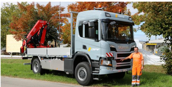
SUR LE SCANIA P500, MANUEL NUNES EXPLOITE UNE GRUE FASSI F255A XE-DYNAMIC DONT LE BRAS HYDRAULIQUE PEUT S'ÉTENDRE JUSQU'À 22.70 MÈTRES.
